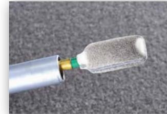
3. Remove the fouling with a clean Bore-tip. Wet with a little solvent and blot dry. Repeat until clean.
