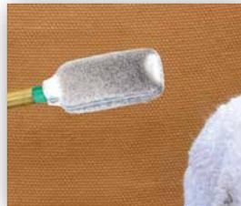
First Squeeze the Bore-tip to blot out any excess solvent or dirt.
