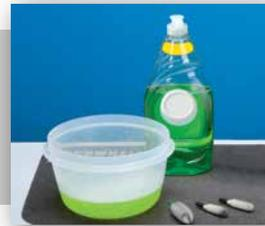
Wash the Bore-tip with a grease cutting soap and warm water. Rinse when clean.
