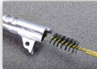
2. Brush the bore to break up any fouling. Apply more solvent if needed.
