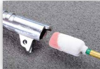
1. Apply a small amount of solvent to a Bore-tip and apply to the barrel. Allow the solvent time to work.
