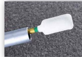
4. Dry the Barrel with a clean bore-tip. You can use another Bore-tip to lubricate the barrel.
